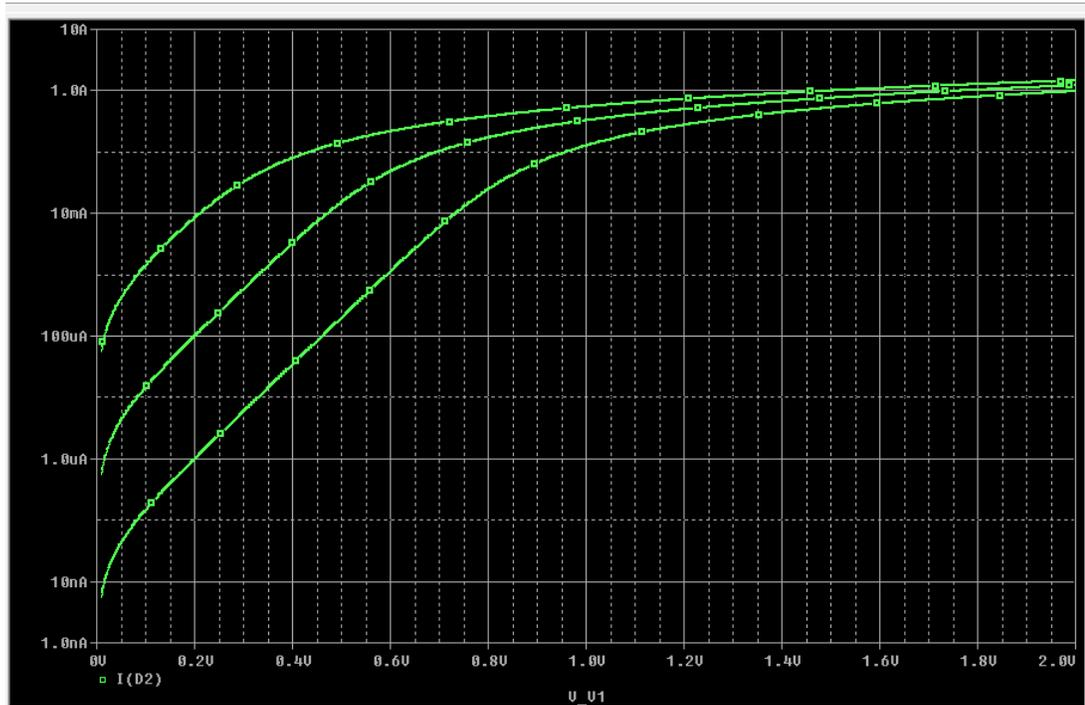
Figure 5: Effect of varying IS parameter value for a schottky diode
