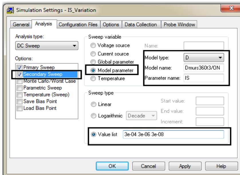
Figure 4: Simulation setting for DC nested sweep- varying model parameter IS
