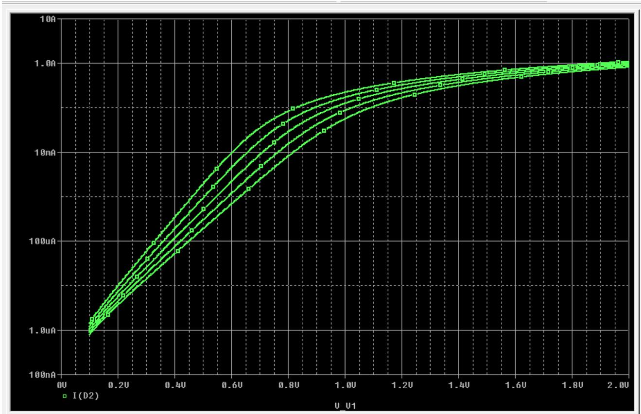
Figure 7: Effect of varying N parameter value for a schottky diode
