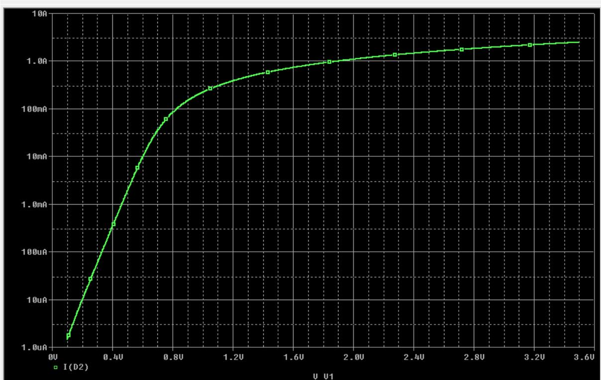
Figure 3: Simulation results –  $IS=3e-07$ ,  $N=2.2$
