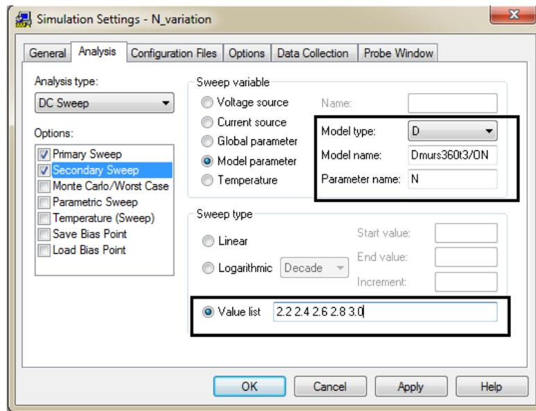
Figure 4A: Simulation setting for DC nested sweep- varying model parameter N
